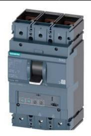
CIRCUIT BREAKER 3VA2 IEC FRAME 630 BREAKING CAPACITY CLASS H ICU=85KA @ 415 V 3-POLE, LINE PROTECTION ETU330, LIG, IN=400A OVERLOAD PROTECTION IR=160A ...400A SHORT CIRCUIT PROTECTION II=1,5...12 X IN GROUND-FAULT-PROTECTION IG=0,2... 1 X IN, TG=0,1/0,3MS BUSBAR CONNECTION
