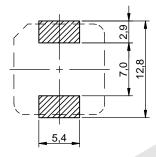
no sensitive traces underneath the component
