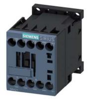
Coupling contactor relay, 2 NO + 2 NC, 60 V DC, 0.7  $\dots$  1.25\* US, with integrated suppressor diode, Size S00, screw terminal suitable for PLC outputs
