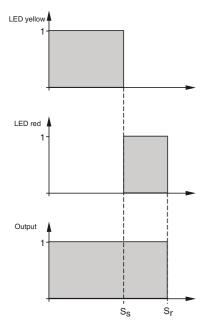
Correlation between output signal/LED-function and stable operating distance s<sub>s</sub>/ effective operating distance  $s_r$ : ( $s_s$  typ. 80 % of  $s_r$ )
