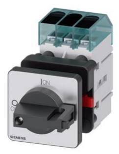
Switch disconnector 3LD3, main switch 3-polig, Iu 25A operational switch at AC-23 A at 400 V 9,0 kW front mounted Base mounting with center-hole 22,5 mm knob-operated mechanism black 48 x 48 mm
