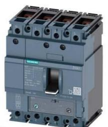
CIRCUIT BREAKER 3VA1 IEC FRAME 160 BREAKING CAPACITY CLASS M ICU=55KA @ 415 V 4-POLE, LINE PROTECTION TM240, ATAM, IN=160A OVERLOAD PROTECTION IR=112A ...160A SHORT CIRCUIT PROTECTION II=5...10 X IN NEUTRAL PROTECTION 100% BUSBAR CONNECTION
