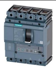
CIRCUIT BREAKER 3VA2 IEC FRAME 100 BREAKING CAPACITY CLASS C ICU=110KA @ 415 V 4POLE, LINE PROTECTION ETU330, LIG, IN=25A OVERLOAD PROTECTION IR=10A ...25A SHORT CIRCUIT PROTECTION II=1,5...12 X IN NEUTRAL PROTECTION ADJUSTABLE(OFF,100%) GROUNDFAULTPROTECTION IG=0,2... 1 X IN, TG=0,1/0,3MS CABLE CONNECTION
