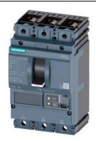
CIRCUIT BREAKER 3VA2 IEC FRAME 160 BREAKING CAPACITY CLASS C ICU=110KA @ 415 V 3POLE, LINE PROTECTION ETU860, LSIG, IN=25A OVERLOAD PROTECTION IR=10A ...25A SHORT CIRCUIT PROTECTION ISD=0,6..10X IN, II=1,5..12X IN NEUTRAL PROTECTION OPTIONAL WITH EXT. CT,UPTO 160% GROUNDFAULT, SWITCHABLE IG=0,2... 1 X IN, TG=0,050,8MS BUSBAR CONNECTION
