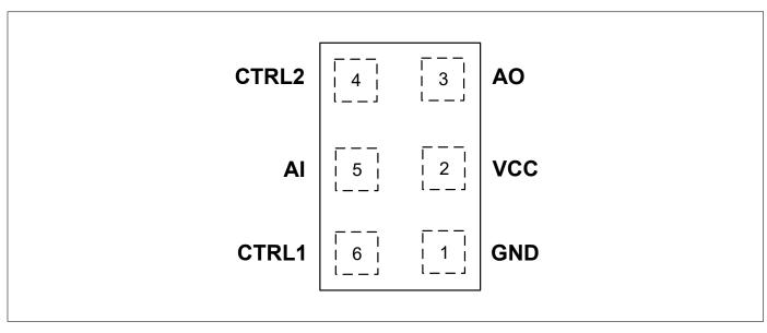
Figure 2: BGA9H1BN6 Pin Configuration (top view)
