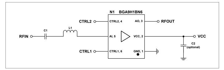
Figure 3: BGA9H1BN6 Application Schematic
