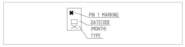
Figure 6: Marking Specification (top view)
