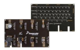
The KITMPXSHOWEVK is conveniently packaged in a padded, embossed plastic case to allow customers to visualize and sample the parts. All of the parts are functional with pads connecting the necessary device pins to the board edge. A simplified pressure converter table is located on the reverse side for quick reference.
