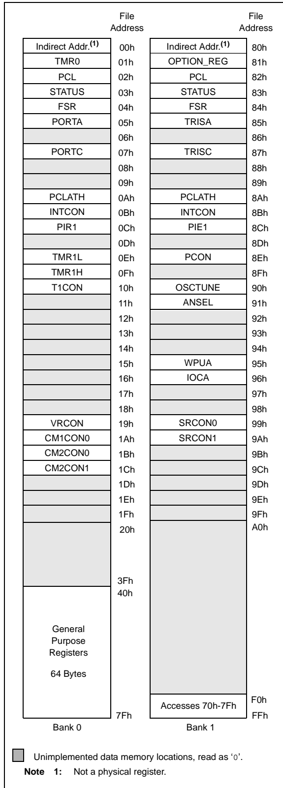
FIGURE 2-3: DATA MEMORY MAP OF THE PIC16F610/16HV610
