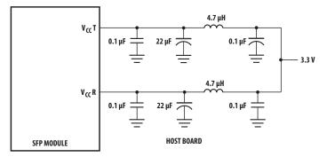
NOTE: INDUCTORS MUST HAVE LESS THAN 1 $\Omega$  series resistance to limit voltage drop to the SFP module.
