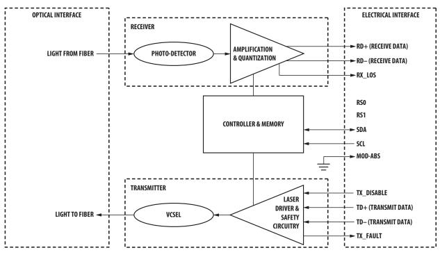
Figure 1. Transceiver functional diagram
