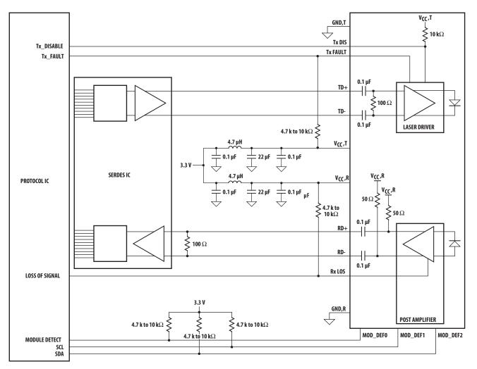
Figure 2. Typical application configuration
