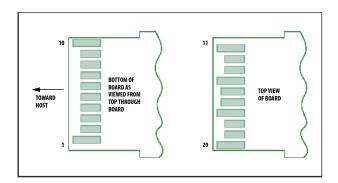
Figure 4. Module edge connector contacts
