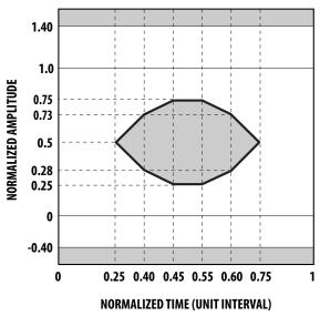
Figure 5a. Receiver Electrical Optical Eye Mask Definition
