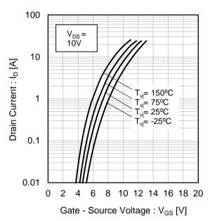
Fig.12 Typical Transfer Characteristics (II)
