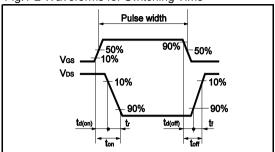
Fig.2-2 Waveforms for Switching Energy Loss
