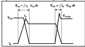
Fig.3-2 Reverse Recovery Waveform
