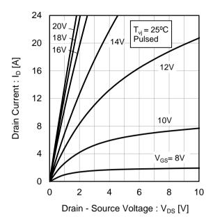
Fig.5 Typical Output Characteristics(II)
