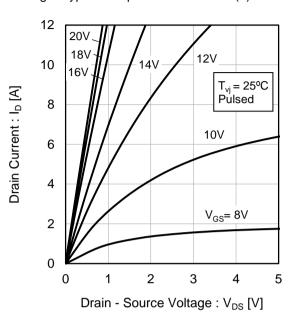
Fig.6  $T_{v_i}$  = 25°C 3rd Quadrant Characteristics
