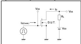
Fig.2-1 Switching Energy Measurement Circuit
