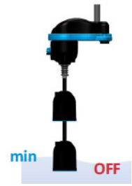
Low level stops the pump
