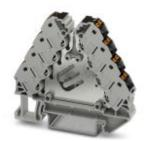
Potential distributors, Nom. voltage: 250 V, Nominal current: 17.5 A, Cross section: 0.14 mm² - 2.5 mm², AWG: 14 - 26, Connection method: Push-in connection, Number of positions: 2, Number of connections: 16, Width: 8.3 mm, Length: 64 mm, Color: gray, Color of connection elements: black, Assembly: NS 35/7,5, NS 35/15
