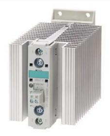
SOLID-STATE CONTACTOR 3RF2,1-PH AC51 40A 40C 48-600V / 4-30V DC SCREW-TYPE TERMINAL BLOCKING VOLTAGE 1200V
