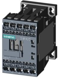
2NO+2NC CONTACTOR, AC3: 5.5KW DC 24V 4-POLE, 2NO+2NC, SZ: S00, SPRING-LOADED TERMINAL
