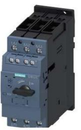
CIRCUIT BREAKER, SIZE S2, FOR MOTOR PROTECTION, CLASS 10, A-RELEASE 20...25A, N-RELEASE 325A, SCREW TERMINAL, STANDARD BREAKING CAPACITY W. TRANSV. AUX. SWITCH 1NO+1NC
