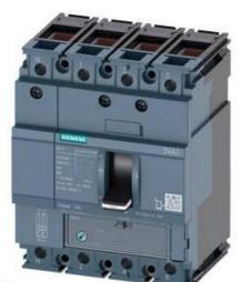
CIRCUIT BREAKER 3VA1 IEC FRAME 160 BREAKING CAPACITY CLASS S ICU=36KA @ 415 V 4-POLE, LINE PROTECTION TM220, ATFM, IN=100A OVERLOAD PROTECTION IR=70A ...100A SHORT CIRCUIT PROTECTION II=10 X IN NEUTRAL PROTECTION 50% CABLE CONNECTION
