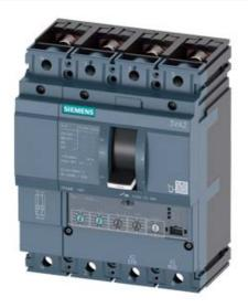
CIRCUIT BREAKER 3VA2 IEC FRAME 160 BREAKING CAPACITY CLASS C ICU=110KA @ 415 V 4POLE, LINE PROTECTION ETU350, LSI, IN=100A OVERLOAD PROTECTION IR=40A ...100A SHORT CIRCUIT PROTECTION ISD=1,5... 10 X IR, II=12 X IN NEUTRAL PROTECTION ADJUSTABLE(OFF,50%,100%) BUSBAR CONNECTION
