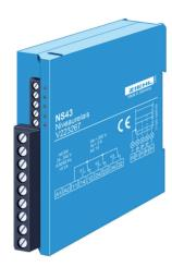
The level monitor NS43 regulates the level of liquid in a container between 2 electrodes. In the normal operation the level of the liquid is situated between the electrodes E2 and E3. The relay K2 tightens, if the level E3 is achieved and drops, if E2 is fallen below. Over the output contacts (1 change-over switch) a pump or a valve can be controlled depending upon case of application and so the level be
