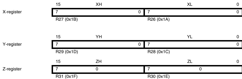
Figure 7-3. The X-, Y-, and Z-registers
