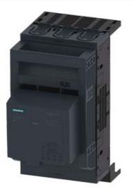
FUSE-SWITCH-DISCONNECTOR 3-POLE, NH00, 160A 40MM BUSBAR SYSTEM COVERS FOR RITTAL FLAT CONNECTOR FUSE MONITORING ELECTRONIC, EFM 10
