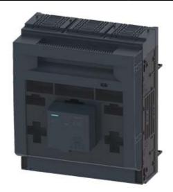
FUSE-SWITCH-DISCONNECTOR 3-POLE, NH3, 630A 60MM BUSBAR SYSTEM COVER LEVEL 32/70 MM FLAT CONNECTOR FUSE MONITORING ELECTRONIC, EFM 10
