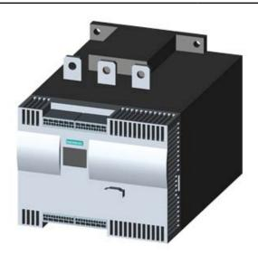
SIRIUS SOFT STARTER, VALUES WITH 460 V, 50 DEG., STANDARD: 280A, 200HP, INSIDE-DELTA CIRCUIT 3: 485A, 400HP, 200-460 V AC, 115 V AC, CAGE CLAMP TERMINALS
