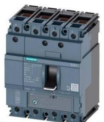
CIRCUIT BREAKER 3VA1 IEC FRAME 160 BREAKING CAPACITY CLASS M ICU=55KA @ 415 V 4-POLE, LINE PROTECTION TM220, ATFM, IN=63A OVERLOAD PROTECTION IR=44,1A ...63A SHORT CIRCUIT PROTECTION II=10 X IN NEUTRAL UNPROTECTED CABLE CONNECTION
