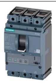
CIRCUIT BREAKER 3VA2 IEC FRAME 100 BREAKING CAPACITY CLASS H ICU=85KA @ 415 V 3POLE, LINE PROTECTION ETU330, LIG, IN=40A OVERLOAD PROTECTION IR=16A ...40A SHORT CIRCUIT PROTECTION II=1,5...12 X IN GROUNDFAULTPROTECTION IG=0,2... 1 X IN, TG=0,1/0,3MS CABLE CONNECTION
