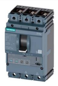
CIRCUIT BREAKER 3VA2 IEC FRAME 160 BREAKING CAPACITY CLASS M ICU=55KA @ 415 V 3POLE, LINE PROTECTION ETU350, LSI, IN=160A OVERLOAD PROTECTION IR=64A ...160A SHORT CIRCUIT PROTECTION ISD=1,5... 10 X IR, II=10 X IN BUSBAR CONNECTION
