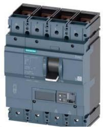
CIRCUIT BREAKER 3VA2 IEC FRAME 400 BREAKING CAPACITY CLASS C ICU=110KA @ 415 V 4-POLE, LINE PROTECTION ETU560, LSIG, IN=250A OVERLOAD PROTECTION IR=100A ...250A SHORT CIRCUIT PROTECTION ISD=0,6..10X IN, II=1,5..12X IN NEUTRAL PROTECTION ADJUSTABLE (OFF, UPTO 160%) GROUND-FAULT, SWITCHABLE IG=0,2... 1 X IN, TG=0,05-0,8MS BUSBAR CONNECTION
