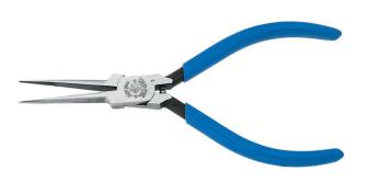
Long, narrow nose and slim hinge for extremely close quarter work. Finely knurled jaws grip thin wire without damaging it. Spring-loaded for self-opening action. Curved handles provide greater tool control.
