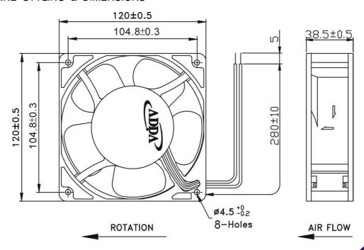
LEAD WIRES: UL 1007, AWG24; L =280±10 mm Red = positive; Black = negative.
