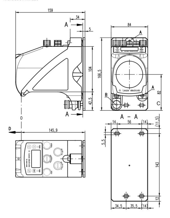
A M 5 screw for alignment
