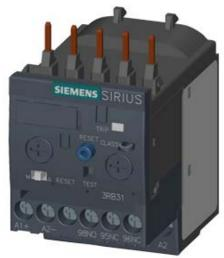
OVERLOAD RELAY 0.32...1.25 A FOR MOTOR PROTECTION SIZE S00. CLASS 5...30 CONTACTOR ASS. MAIN CIRCUIT: SCREW CONN. AUX.CIRCUIT: SCREW CONN. MANUAL-AUTOM.-RESET INT. GROUND FAULT DETECTION
