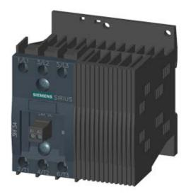
SOLID-STATE CONTACTOR 3-PH 3RF3 AC53 9.2A 40 DEGREES C 48-480V / 24V DC 2-PH. CONTROLLED INSTANTANEOUS SCREW TERMINALS
