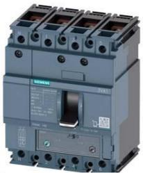
CIRCUIT BREAKER 3VA1 IEC FRAME 160 BREAKING CAPACITY CLASS S ICU=36KA @ 415 V 4-POLE, LINE PROTECTION TM240, ATAM, IN=25A OVERLOAD PROTECTION IR=17,5A ...25A SHORT CIRCUIT PROTECTION II=5...10 X IN NEUTRAL UNPROTECTED BUSBAR CONNECTION
