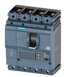
CIRCUIT BREAKER 3VA2 IEC FRAME 100 BREAKING CAPACITY CLASS C ICU=110KA @ 415 V 4POLE, LINE PROTECTION ETU550, LSI, IN=63A OVERLOAD PROTECTION IR=25A ...63A SHORT CIRCUIT PROTECTION ISD=0,6..10X IN, II=1,5..12X IN NEUTRAL PROTECTION ADJUSTABLE (OFF, UPTO 160%) BUSBAR CONNECTION
