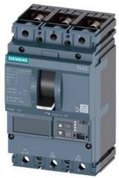
CIRCUIT BREAKER 3VA2 IEC FRAME 160 BREAKING CAPACITY CLASS C ICU=110KA @ 415 V 3POLE, LINE PROTECTION ETU550, LSI, IN=40A OVERLOAD PROTECTION IR=16A ...40A SHORT CIRCUIT PROTECTION ISD=0,6..10X IN, II=1,5..12X IN NEUTRAL PROTECTION OPTIONAL WITH EXT. CT,UPTO 160% BUSBAR CONNECTION
