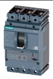
CIRCUIT BREAKER 3VA2 IEC FRAME 250 BREAKING CAPACITY CLASS L ICU=150KA @ 415 V 3POLE, LINE PROTECTION ETU330, LIG, IN=250A OVERLOAD PROTECTION IR=100A ...250A SHORT CIRCUIT PROTECTION II=1,5...10 X IN GROUNDFAULTPROTECTION IG=0,2... 1 X IN, TG=0,1/0,3MS BUSBAR CONNECTION
