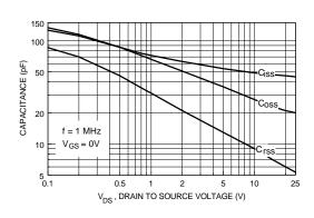
Figure 8. Capacitance Characteristics.
