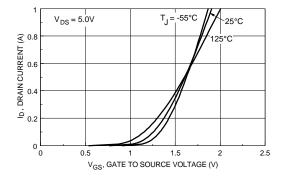
Figure 5. Transfer Characteristics.
