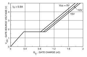
Figure 7. Gate Charge Characteristics.
