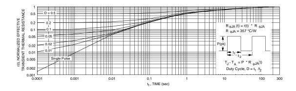
Figure 11. Transient Thermal Response Curve.
