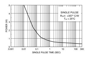
Figure 10. Single Pulse Maximum Power Dissipation.
