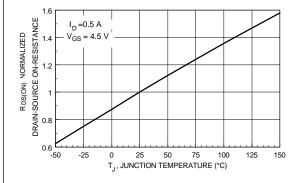
Figure 3. On-Resistance Variation with Temperature.
