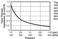
Thermal impedance reduces significantly with pressure, ensuring excellent performance in pressure ranges common for most standard modules and power electronic devices per manufacturer's application guide.
