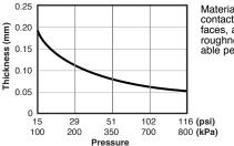
Material compressibility improves contact between the mating surfaces, adjusting for flatness and roughness variations, ensuring reliable performance.
