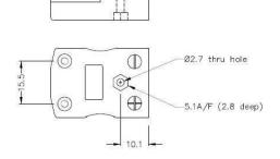
Standard in-line Plug (dimensions in mm)
