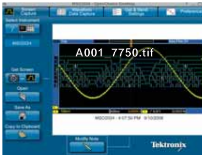
OpenChoice® Desktop - Standard software seamlessly connects the oscilloscope to a PC.
