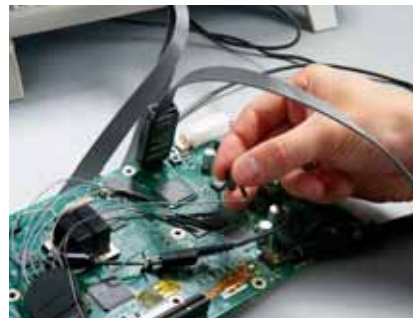
The P6316 digital probe for MSO2000 Series simplifies connection to the device-under-test
