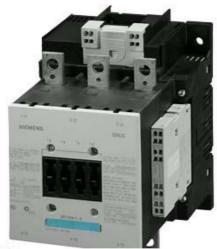
CONTACTOR, 90KW/400V/AC-3 AC(40...60HZ)/DC OPERATION UC 23-26V AUXILIARY CONTACTS 2NO+2NC 3-POLE, SIZE S6 BAR CONNECTIONS CONVENT. OPERATING MECHANISM CAGE CLAMP TERMINAL
