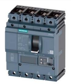
CIRCUIT BREAKER 3VA2 IEC FRAME 100 BREAKING CAPACITY CLASS H ICU=85KA @ 415 V 4POLE, LINE PROTECTION ETU860, LSIG, IN=40A OVERLOAD PROTECTION IR=16A ...40A SHORT CIRCUIT PROTECTION ISD=0,6..10X IN, II=1,5..12X IN NEUTRAL PROTECTION ADJUSTABLE (OFF, UPTO 160%) GROUNDFAULT, SWITCHABLE IG=0,2... 1 X IN, TG=0,050,8MS BUSBAR CONNECTION
