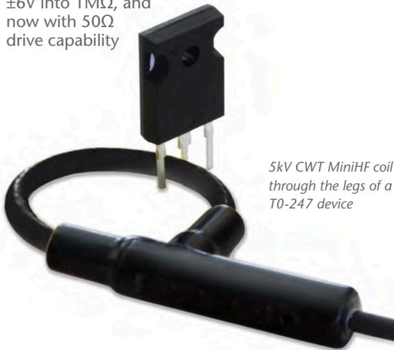
5kV CWT MiniHF coil through the legs of a TO-247 device
