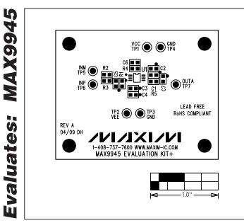
Figure 2. MAX9945 EV Kit Component Placement Guide— Component Side
