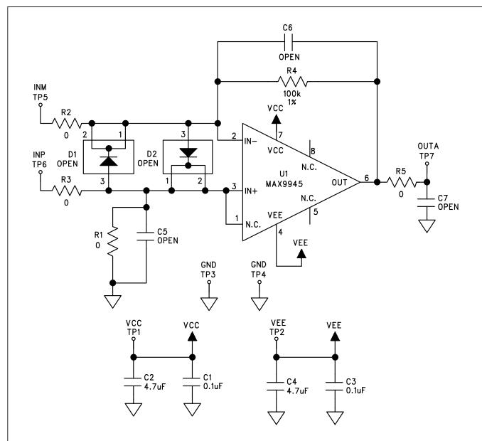
Figure 1. MAX9945 EV Kit Schematic
