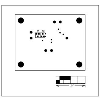
Figure 5. MAX9945 EV Kit Component Placement Guide—Solder Side
