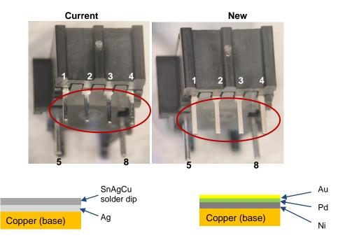
Active pins (pin1 to pin4 in red circle): Affected by changing to new NiPdAu lead-frame finish. Housing staple pins (pin5 and pin8): No Change.
