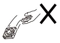
Don't cut the fan or lead wires
