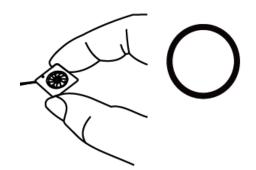
Don't pull fan with lead wires.
