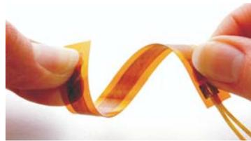
**Thermistor:** A temperature sensor made from semiconductive material. Thermistors are highly sensitive (resistance changes dramatically with temperature), but non-linear and typically not very accurate.
