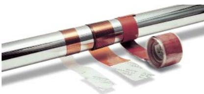
Built-to-order shrink bands are pre-stretched strips of film with adhesive coated ends. Wrap around the heater and heat to shrink. Stretch tape installs quickly with no heat required.
