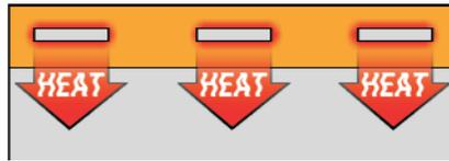
Proper installation ensures good heat flow from the heater to the heat sink
