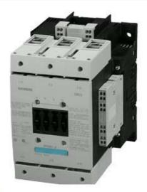
CONTACTOR, 55KW/400V/AC-3 AC(40...60HZ)/DC OPERATION UC 220-240V AUXILIARY CONTACTS 2NO+2NC 3-POLE, SIZE S6 WITH BOX TERMINALS CONVENTIONAL OPERATING MECHAN. CAGE CLAMP CONNECTION
